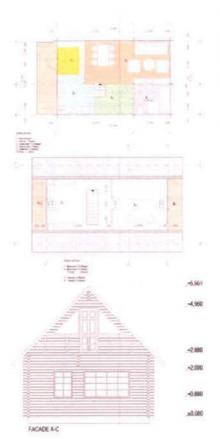
Dimensions: 5.90x8.90 m Wall thickness 68mm Double glazed windows Includes the floor in 28mm T&G Roof area : 110m2, Double roof: inside 20mm thickness, outside plywood. Ridge height overall:
